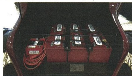
A 1917 Milburn electric car was on display at the Classics & Chrome Auto Show this past weekend in Machesney Park. The car featured a battery driven motor, with the power supply housed in its trunk. Photos, Allen Penticoff
